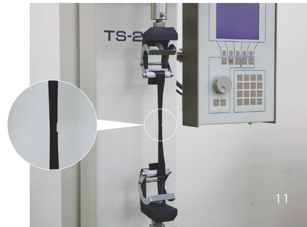
Tear strength test (crescent piece)
