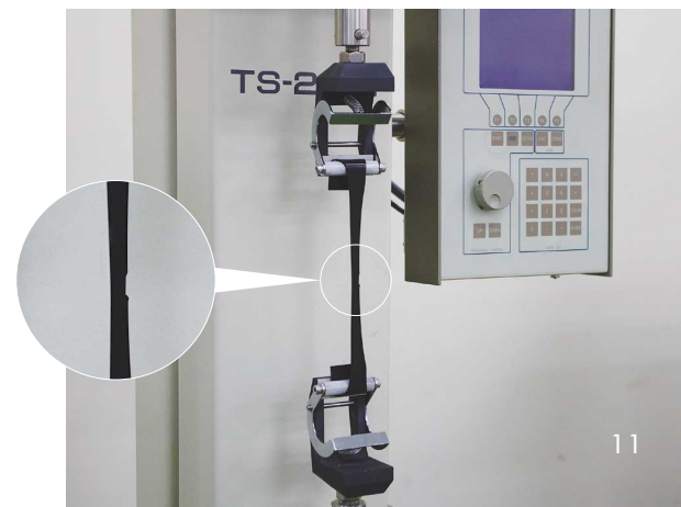
Tear strength test (crescent piece)
